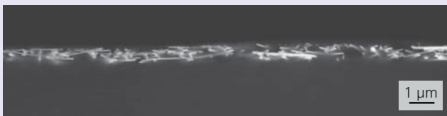
SEM image of PET foil with embedded silver nanowires
