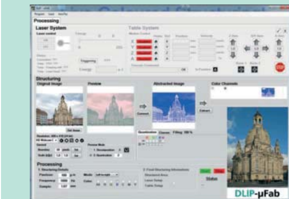
Software tool for DLIP system control and transfer of bitmap images
